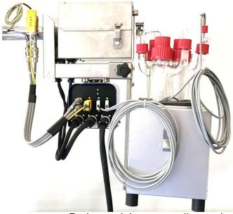
Probe module on sampling probe
